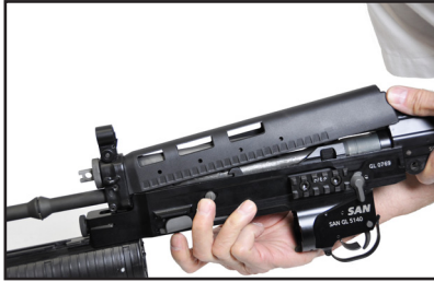
Fig. 8: Install upper hand guard
