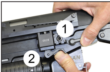
Fig. 9: Excentric latch in horizontal position (1)
