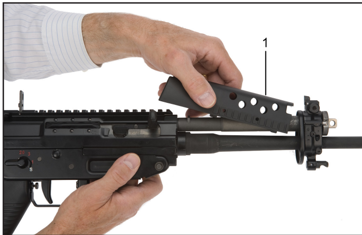
Figure 4: Install upper hand guard for GL 5340
