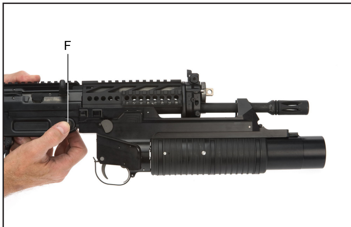
Figure 9: Press in front trigger casing stud
