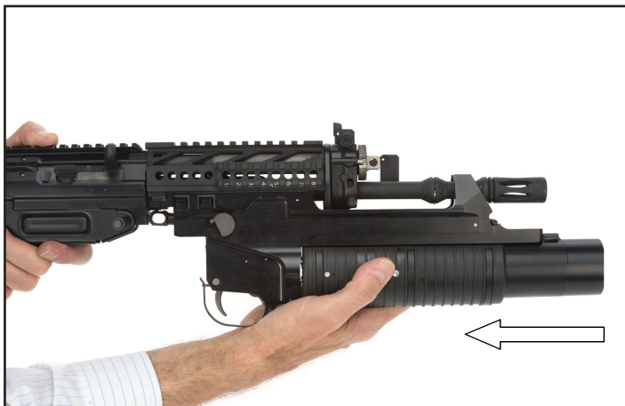
Figure 8: Draw back the GL 5340 as far as the stop
