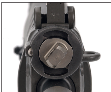
Figure 38: Gas valve in position II
