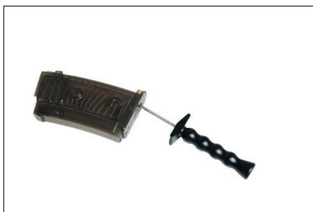
Figure 56: Stripping the magazine
