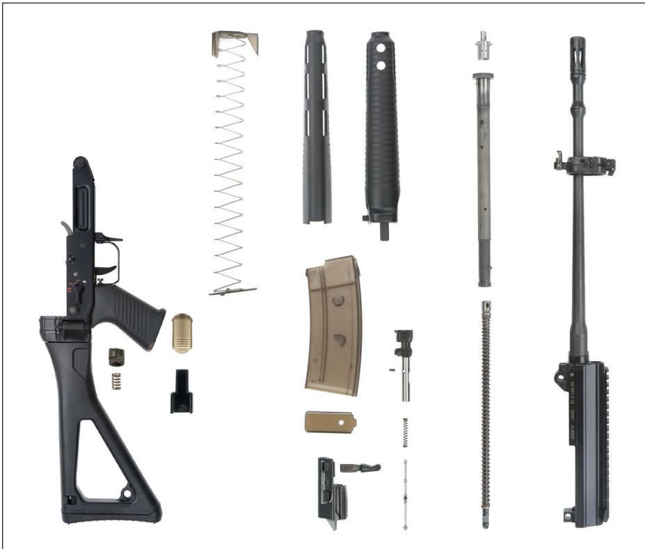
Figure 59: SG 551 LB Picatinny version stripped
