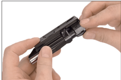
Figure 50: Remove bolt head (rotate)
