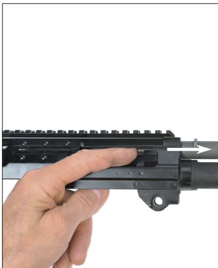
Figure 54: Remove gas piston
