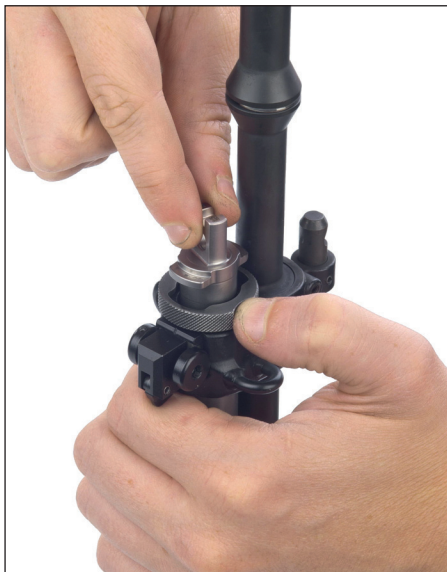
Figure 53: Remove gas valve
