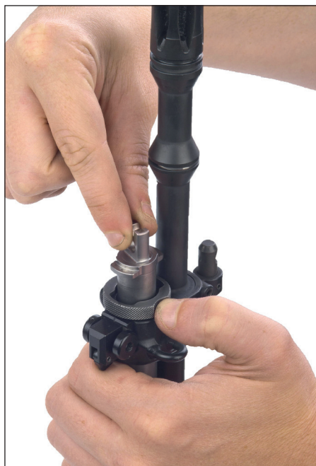
Figure 63: Install gas valve
