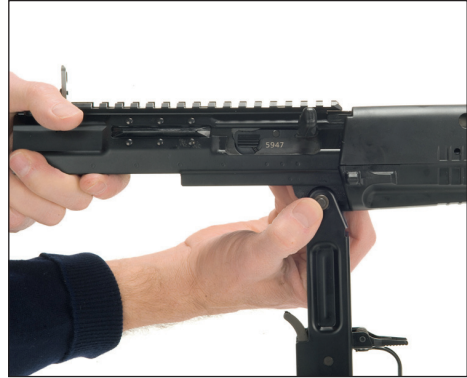
Figure 47: Remove trigger assembly
