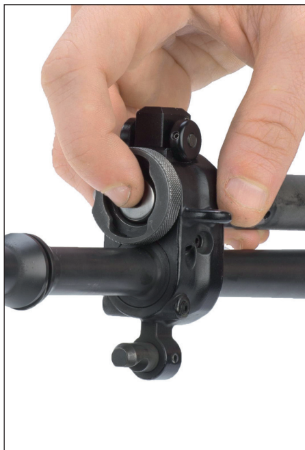
Figure 62: Check gas piston position
