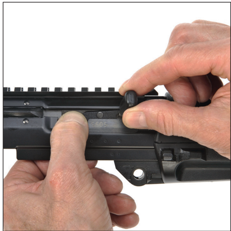
Figure 48: Remove charging handle
