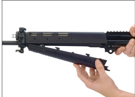
Figure 52: Lift off lower handguard
