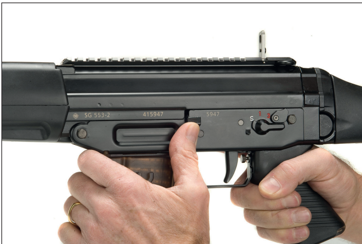
Figure 27: Push the bolt catch up
