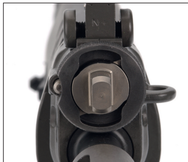
Figure 37: Gas valve in position I
