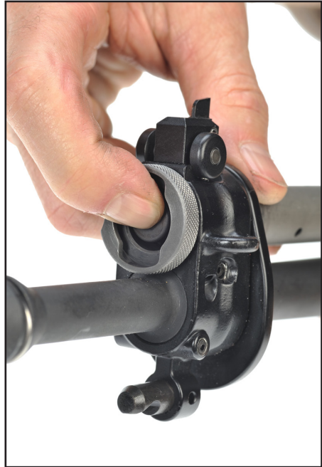
Figure 62: Check gas piston position
