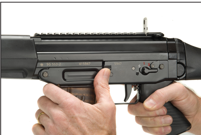
Figure 27: Push the bolt catch up
