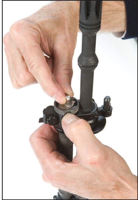
Figure 63: Install gas valve
