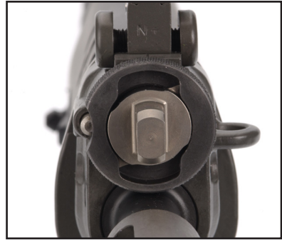
Figure 37: Gas valve in position I
