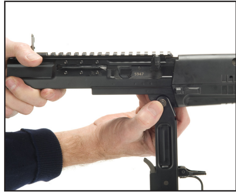
Figure 47: Remove trigger assembly
