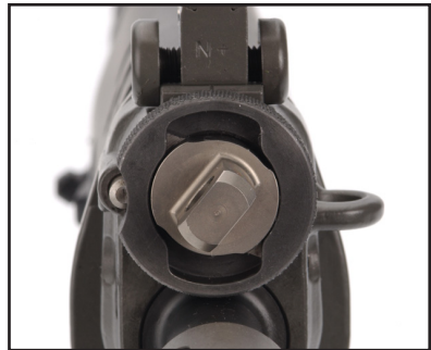
Figure 38: Gas valve in position II
