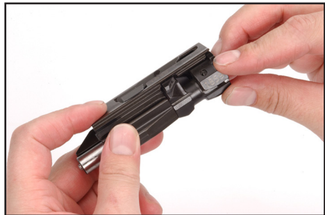
Figure 50: Remove bolt head (rotate)
