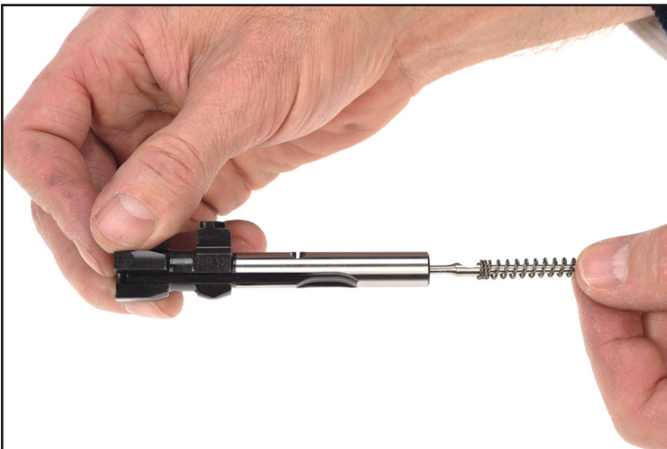
Figure 61: Install firing pin
