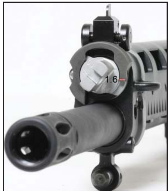
Figure 22: Gas valve position II
