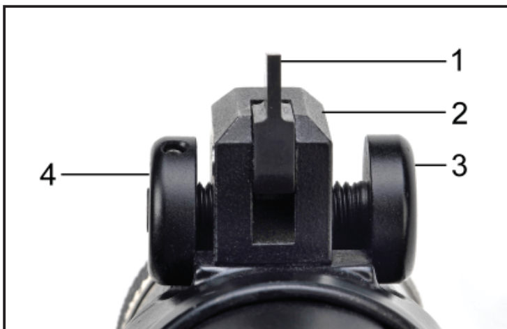
Figure 13: Flip up front sight
