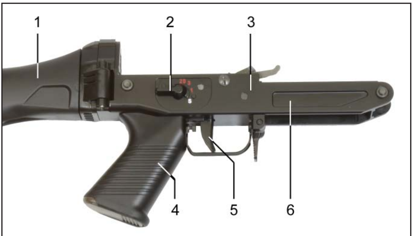
Figure 10: Trigger assembly and butt stock from right
