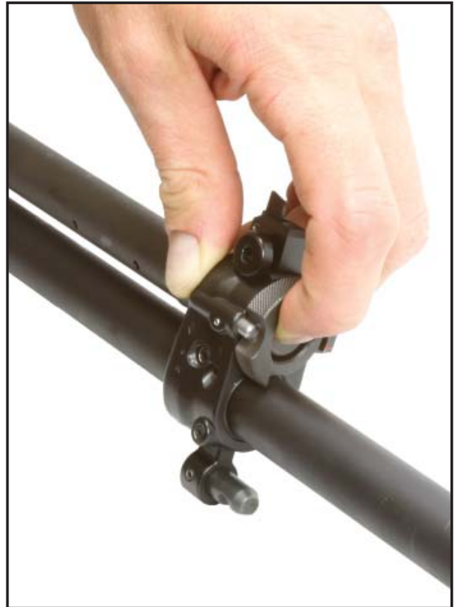
Figure 44: Install gas tube
