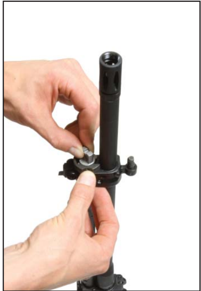
Figure 45: Install gas valve
