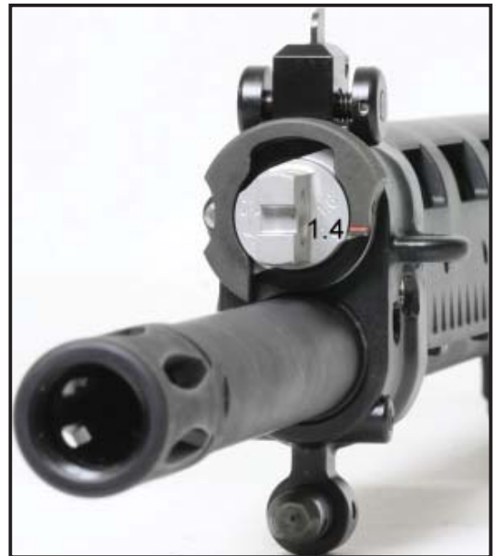
Figure 21: Gas valve position I
