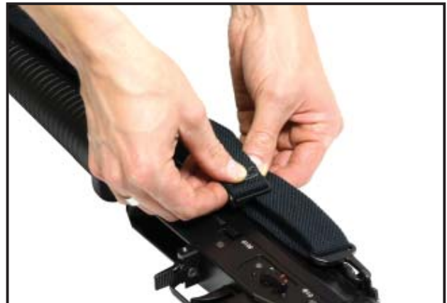
Figure 29: Fix the taut sling
