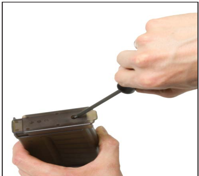
Figure 40: Stripping the magazine
