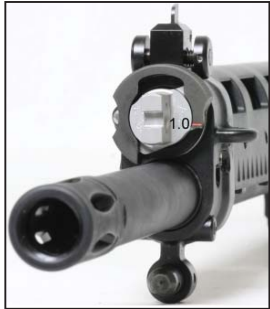
Figure 23: Gas valve position III
