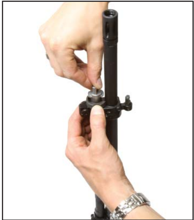
Figure 37: Remove gas valve
