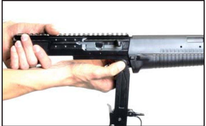
Figure 31: Remove trigger assembly
