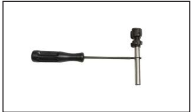
Figure 39: Remove firing pin
