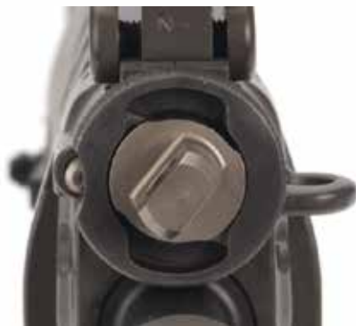
Figure 38: Valve de gaz en position II
