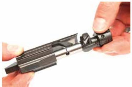
Figure 51: Enlever la culasse (traction)
