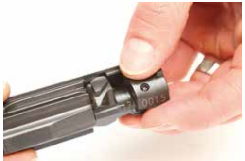
Figure 50: Enlever la culasse (rotation)
