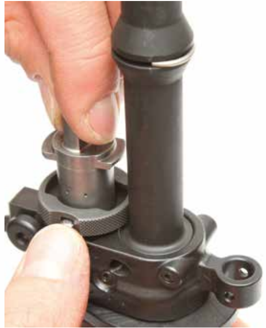
Figure 53: Enlever la valve de gaz
